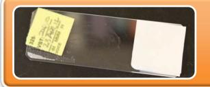
Correct SCHARP label used but on wrong end of the slide
