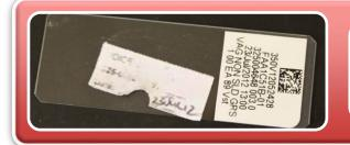
Incorrect labels used & labels placed directly on top of specimens
